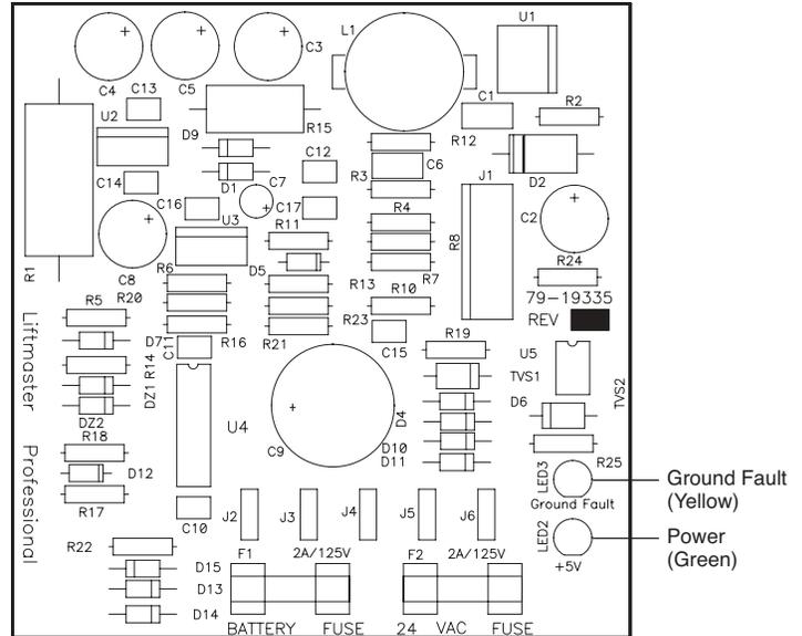
Figure 2 - Power Supply Board LED Descriptions
