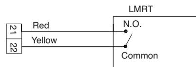
**NOTE:** LMRT key switch must be installed within a single gang junction box with a minimum 2" depth using appropriate 6-32 mounting screws and mounted on the same wall and within the same room as is the release device. All wire connections must be secured with appropriate wire nuts.
