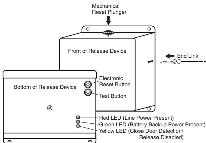
After completing all tests, make sure the door is in its normal position (open or closed) and all power required for normal operation is restored to unit. The release device is designed to operate with power applied.
